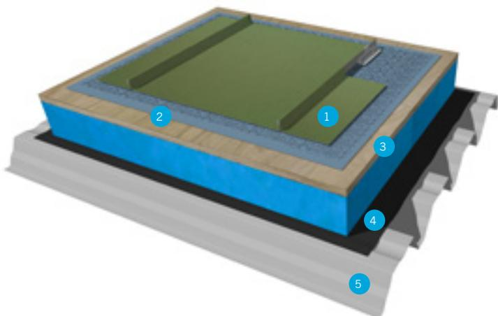
**Warm roof – timber insulating board**
