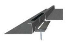
Self-expanding sealing strip on undercloak
