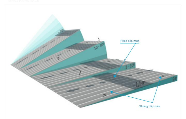
The distribution of the fixed clips depends on roof pitch – the steeper the pitch, the higher the band of fixed clips is positioned. This means that the lower the pitch of the roof, both the longer the trays can be before an expansion joint must be introduced or before special measures need to be taken, for example the use of special sliding clips.
