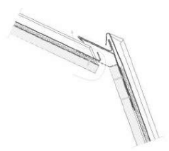
Vented transition mansard roof
